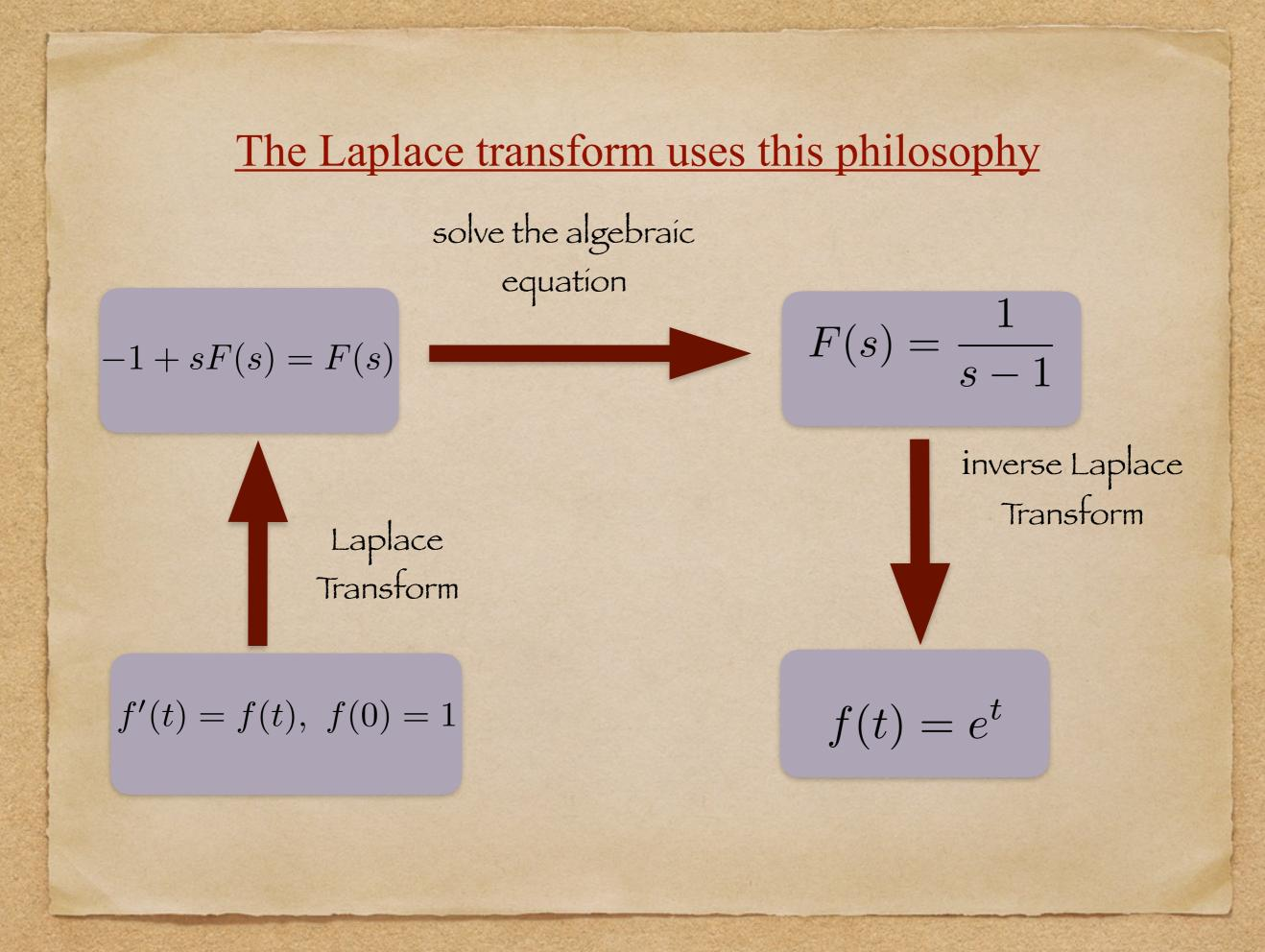
What is not revealed by this diagram is how to pass from the original equation
