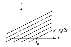
• The initial data is propagated along the projected characteristic curves. For this reason, (2.3) is known as the transport equation. Information is simply propagated along lines.
