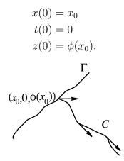
If we construct a characteristic curve from each point on  $(\Gamma, \phi)$  and take the union of these characteristic curves, we can find an integral surface S for the vector field (a, 1, 0) which contains the curve  $(\Gamma, \phi)$ . This integral surface will give us a solution to (2.5).
