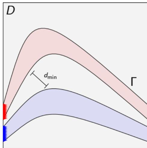
$$\min_{\Gamma} \quad J(\Omega_f) = - \left( \int_{\Omega_{f,cold}} \rho c_p \mathbf{v} \cdot \nabla T dx - \int_{\Omega_{f,hot}} \rho c_p \mathbf{v} \cdot \nabla T dx \right)$$
