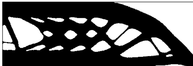
(c) Optimized shape with maximum thickness constraint.
