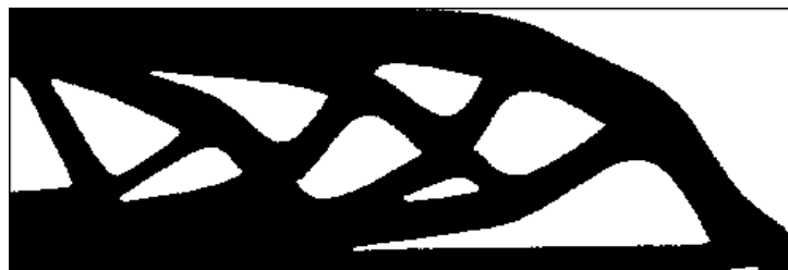
(c) Optimized shape with minimum thickness constraint ( d_{\min} = 0.2 ).
