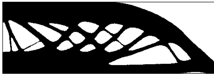
(a) Optimized shape without minimum thickness constraint.
