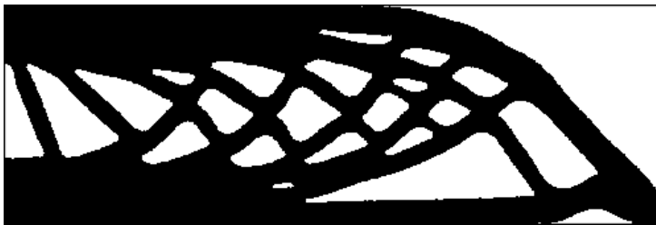
(b) Optimized shape with minimum thickness constraint ( d_{\min} = 0.1 ).
