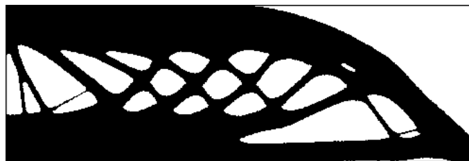
(b) Optimized shape without maximum thickness constraint ( \max d_{\Omega} = 0.36 ).
