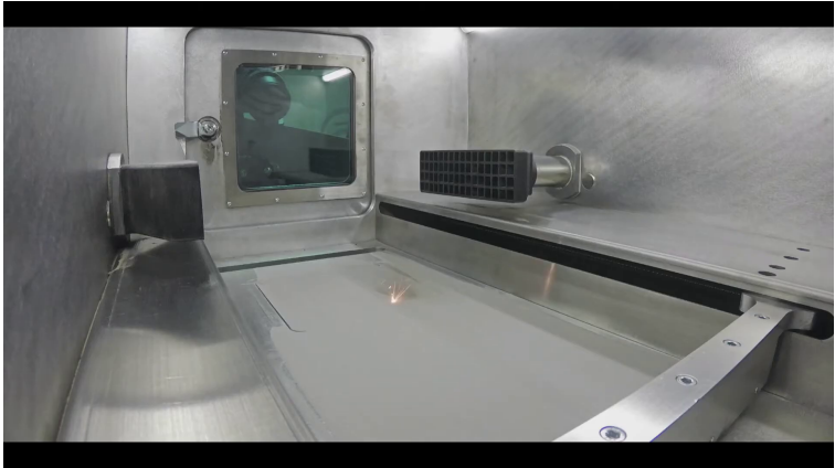
Figure: Additive manufacturing: metal powder bed fusion (source: https://www.youtube.com/watch?v=Y-dTc8_3dU0 ).
