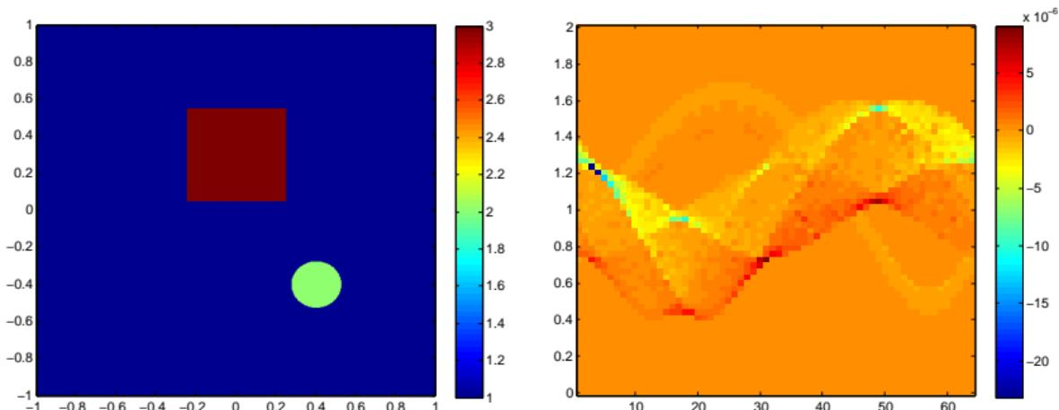
True absorption (left) and measurements  $M_u$  (right)
