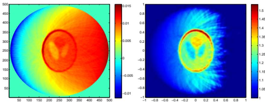
Reconstruction of the Shepp-Logan phantom for 128 acoustic pulses.
