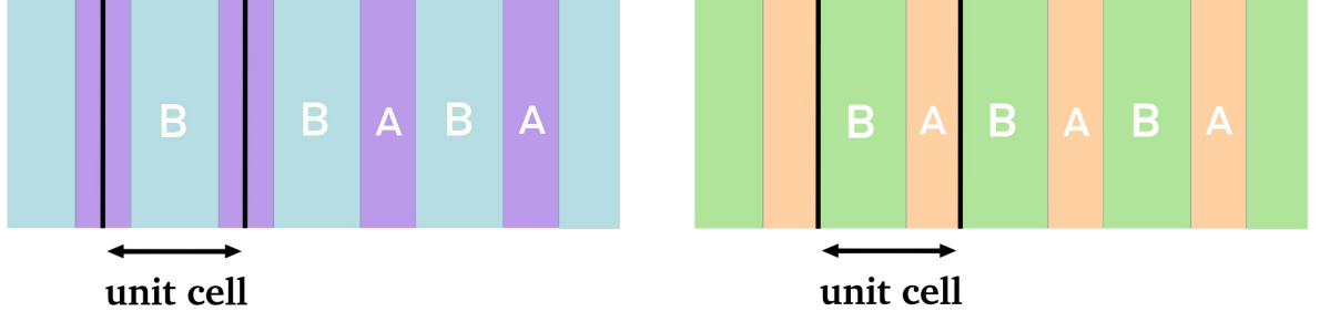
Figure 3: Inversion-symmetric and non-symmetric unit cell
