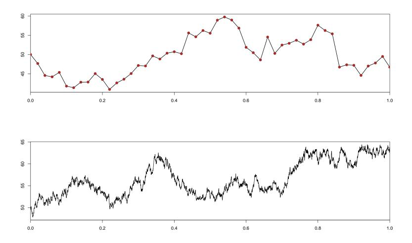
Euler discretization of the SDE  $dS(t) = S(t)(\mu dt + \sigma dW(t))$  with  $S_0 = 50$ ,  $\mu = 0.05$ ,  $\sigma = 0.3$ , and time increments  $\Delta t = 1/50$  (upper graph) and  $\Delta t = 1/5000$  (lower graph)
