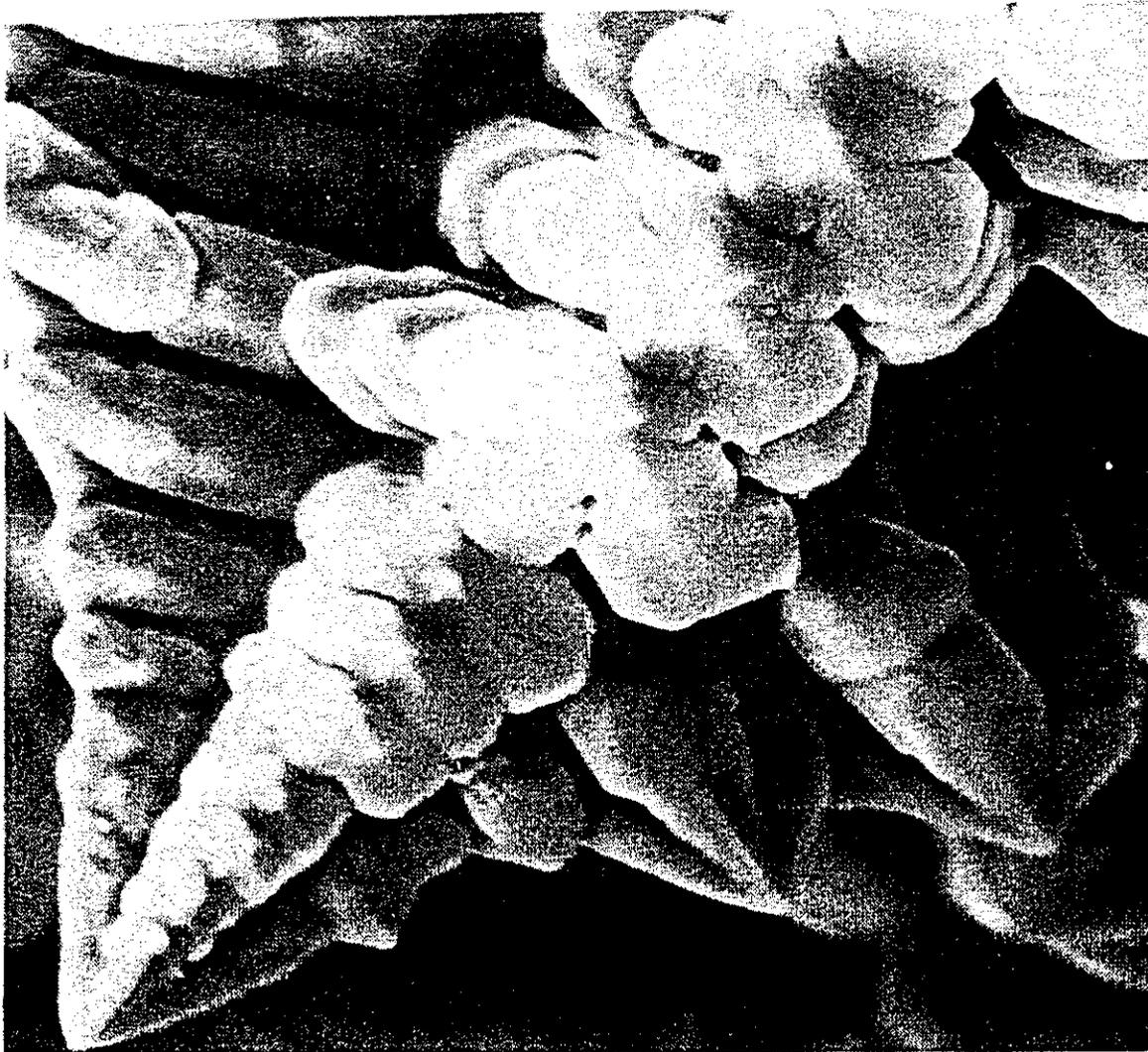
Dendritic growth shape of icosahedral AlLiCu. Notice the pentagonal section the main dendrite, and of the side structures (courtesy of CECM-CNRS, Vitry).
