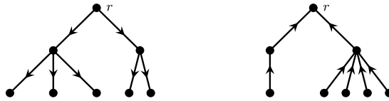
Fig. 7. An out-directed tree and an in-directed tree.
